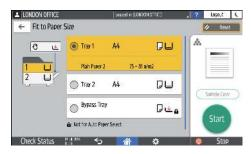
When the orientations of the original and paper in the paper tray do not match, the machine rotates the copied image automatically. To reduce an original of A3 (11 × 17) size to A4 (8 $^{1}/_{2}$  × 11) size, for example, you can select either A4 (8 $^{1}/_{2}$  × 11) $\Box$  or A4 (8 $^{1}/_{2}$  × 11) $\Box$ .
